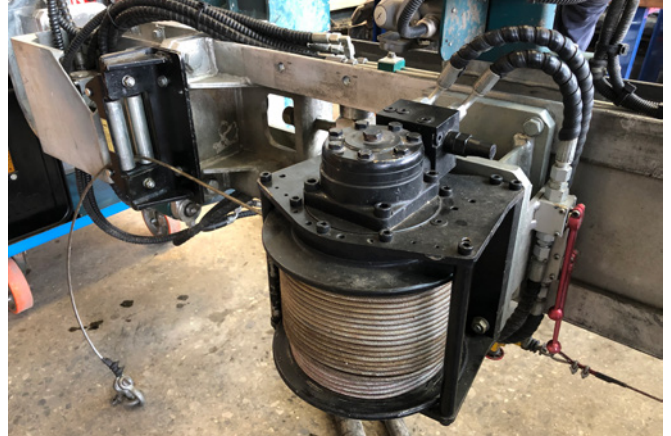
Cable winch mounted to the underside of the drill feed
