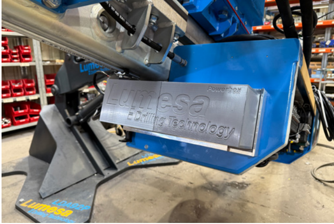
Powerbox (control voltage)
