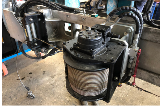
Cable winch mounted to the underside of the drill feed
